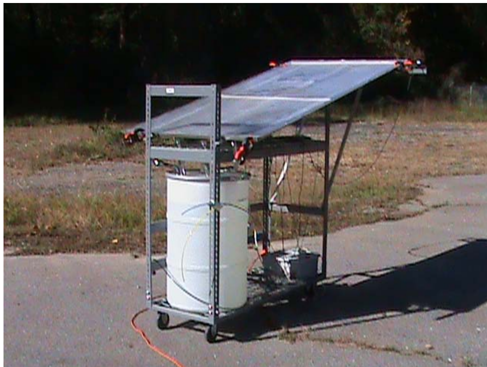
Figure 3-4. A photo of the test set-up for solar UVPCO water treatment system on wheels built by SWA.
