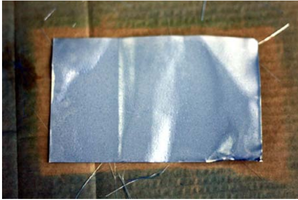
Figure 4-14. Aluminum foil substrate and fiberglass substrate after coated with Methylene Blue dye.
